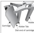
Then push the top 4. part of the cartridge in until it snaps into place
